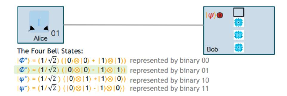
Step 5: Perform a Correction Operation on the Received Qubit (if necessary)
