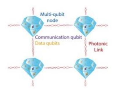
An Example of Optical Quantum Memory Using Engineered Diamonds
